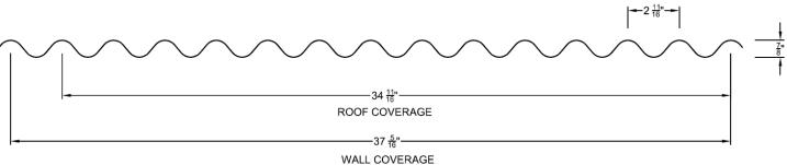
The 7/8" Wave panel provides 37-5/16 inch wall and 34-11/16 inch roof coverage and is composed of major S-shaped ribs at 7/8 inches tall and 2-11/16 inch on center. This product can be utilized as a roofing, liner and/or siding panel. Most commonly it is utilized as an accent or wainscot panel for interior and exterior walls.
