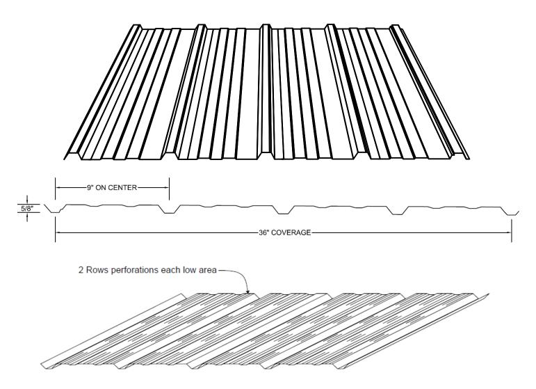
The soffit or inverted panel covers 36 inches and is composed of five inverted ribs at 5/8 inches tall and 9 inches on center. The stiffener ribs between the major ribs are symmetrical with the flat areas to provide an attractive appearance. Vented Soffit provides 9.64 square inches of airflow per one lineal foot. This panel can also be used as an inverted siding panel.
