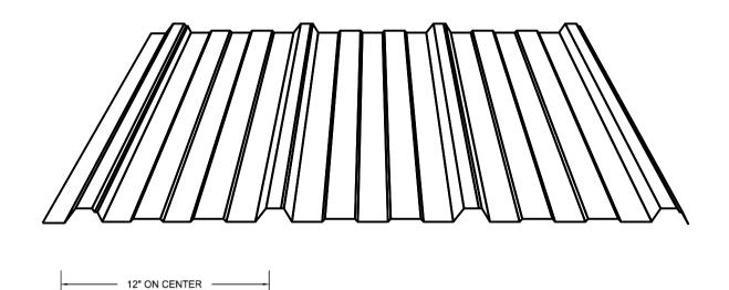
The Husky panel covers 36 inches and is composed of four major ribs at 3/4 inches tall and 12 inch on center. The stiffener ribs between the major ribs are symmetrical with the flat areas to provide an attractive appearance. This product can be utilized as a roofing, liner and/or siding panel.
